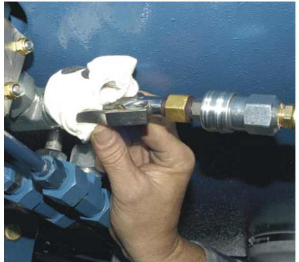
Figure 4: How To Apply Air Pressure to Seals
